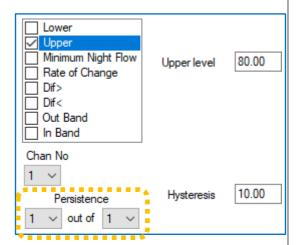
However, if the data from the channel has any possibility of "blips" (spikes or other noise characteristics) the use of the **persistence** settings can be employed to ensure (add greater certainty) that the trigger threshold has been crossed. This is, however, at the expense of delaying the alarm message; it is the nature of the assessment process.
