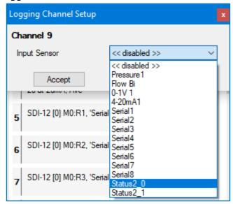
The "\_0" and "\_1" refers to the specific pin being used on the logger interface connector; refer to your logger user-guide for details of pin number or wire-color of any HWM-supplied cable.
