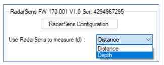
When Depth is selected, IDT requires additional information about the chamber and sensor position. Measure from the bottom of the water channel (or Riverbed, or the internal base of a fluid containment vessel) to the lower face of the installed RadarSens. (Re-check and adjust if the sensor position is ever adjusted).
