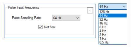
Ensure the logger can capture pulses that are generated at the *maximum* expected meter output rate.
