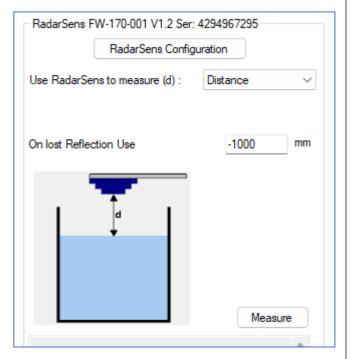
Next, set up the logger to handle the datapoint stream for situations where the RadarSens is unable to detect a reflection signal of any significance. These are known as 'lost reflections'. (Typically, this will be due to a sensor which has not been correctly tuned to the site, or if the channel is dry and unreflective).
