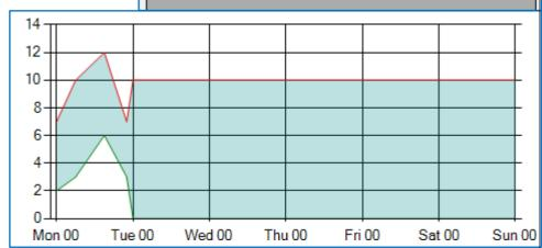
If a step change is needed, create additional lines within the table to ramp up or down to the new value in a short time, maybe a few seconds after the change is required.
