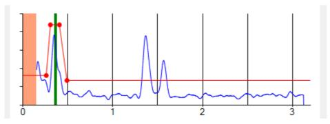
Re-start the sampling to check that the correct reflection is now being selected, and that the nuisance reflection (even if higher) is being disregarded.
