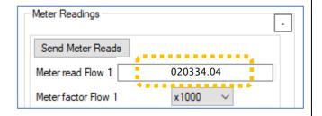
After waiting for the meter to change by a few digits, note the meter reading and re-read the logger to refresh the meter reading values held by IDT.
