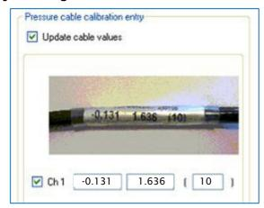
Note: Entry of calibration coefficients (cable values) is the recommended method of entering calibration settings, whenever available.
