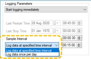
Most logger applications require the measurement interfaces to be logged frequently. For these, set to "Log data at specified time interval".
