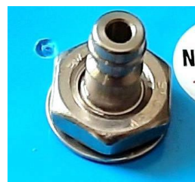
Figure 11. Connection to internal water pressure transducer
