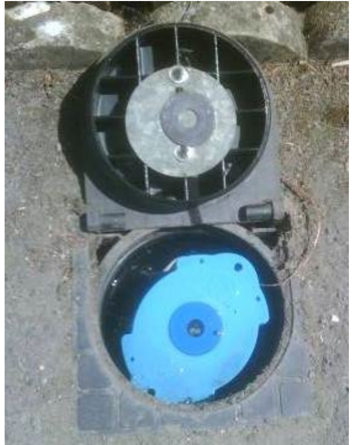
Figure 16. Logger mount using a plastic tube example
