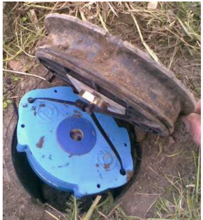
Figure 15. Logger in Talbot flip-lid box P-clip example
