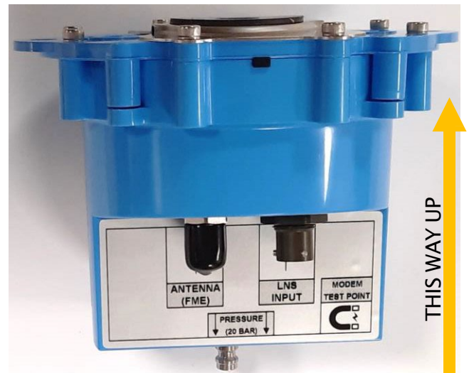
Figure 2. Side view of example logger. Shows interface connectors and labels. Shows correct orientation for best battery life.
