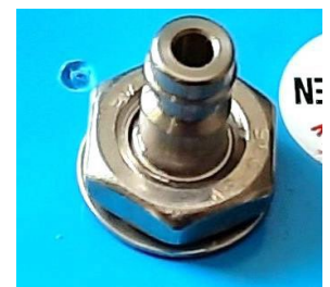
Figure 9. Connection to an internal water pressure transducer
