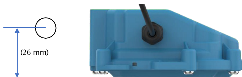
Figure 6. Offset (typical) of RadarSens from center of bracket arm (round)
