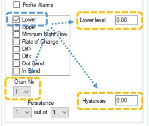
The relevant channel(s) have to be selected within the tab. The channels must have previously been set up and also saved to the logger; if not, they are unavailable for selection.
