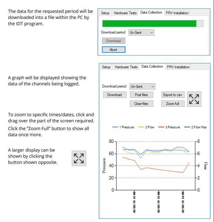
Note: The graph contents will vary according to the sensors attached to the logger, the type of data produced, how long the logger has been running and other factors.
