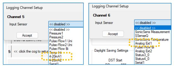
Note: When Analog Ext[n] is selected, it is usually associated with some additional interface unit for the logger (e.g. ESIB series for Intelligens loggers). The logger communicates with the interface unit to determine what type it is; In this case, a 4-20mA unit is being used.
