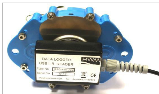
Figure 6. IR Reader coupled to the logger for communications.
