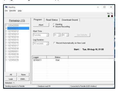
**IMPORTANT**: For accurate correlation of sound recordings, the loggers <u>must</u> be programmed together at the same time, and <u>not</u> separately. The loggers can be programmed and downloaded separately, but this will introduce an error of typically 5m per minute of time difference.
