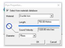
Select the material the pipe is made from, the length of the pipe, and the diameter of the pipe. Click OK.
