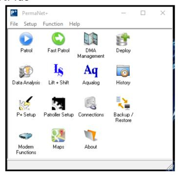
The **Main Screen** contains a set of icons that will lead to the different functions of the PermaNetPlus software. They can also be accessed by the Function menu.
