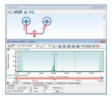
The correlation window will display the results from the correlation algorithms and the probable location of a possible leak.
