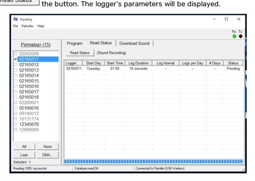
A logger with "--" in the columns "Log Interval", "Logs per Day", and "# Days" has been previously programmed for Sound Recording. Otherwise, it has been programmed for Aqualog.
