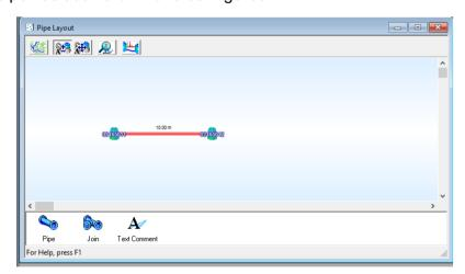
**Note:** It is not necessary for the pipe layout to be a 1:1 scale. The pipes' lengths are set in the Pipe Properties box upon drawing a pipe, and can be changed by right-clicking on the pipe, and selecting "Pipe Properties".
