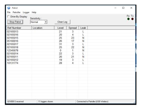
**Note**: for the Patroller unit (whether mobile or USB) to detect the logger, the radio frequencies of Patroller or USB transceiver must match.
