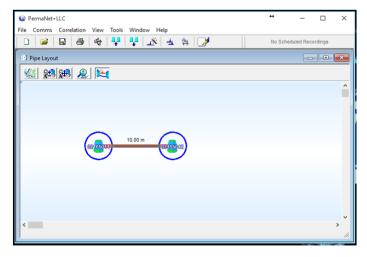
The software will cross-correlate the data from the two loggers, and display the estimated location of a possible leak in the correlation window.
