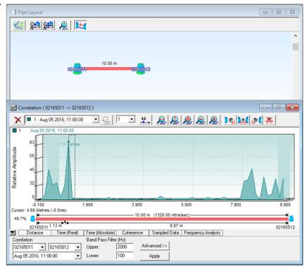
As the text and numbers under the graphical data is in black, the software has concluded it is not a leak.
