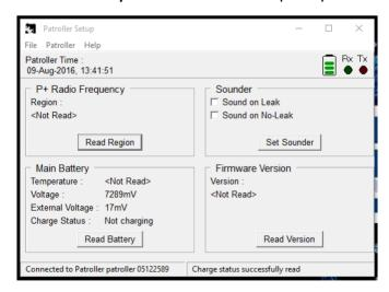
Clicking the Read Region button will detect the operating radio frequency, and therefore the area which the loggers and Patroller unit are in use.
