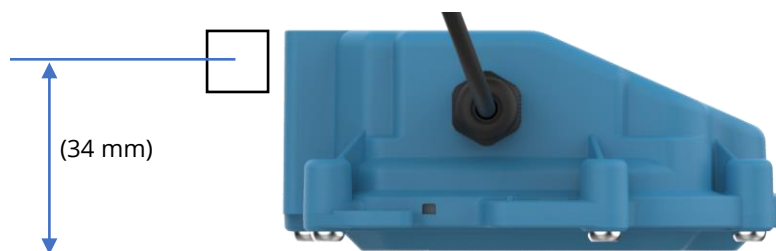
Figure 6. Offset (typical) of RadarSens from center of bracket arm (square)
